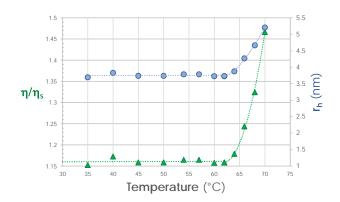
Monitor stability of proteins to determine denaturation or melting temperature by tracking relative viscosity  $(\eta/\eta_s)$  and hydrodynamic radius  $(r_b)$ .
