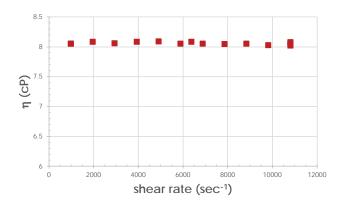
Or determine the impact of shear strength on the sample's microstructure with a shear rate sweep.
