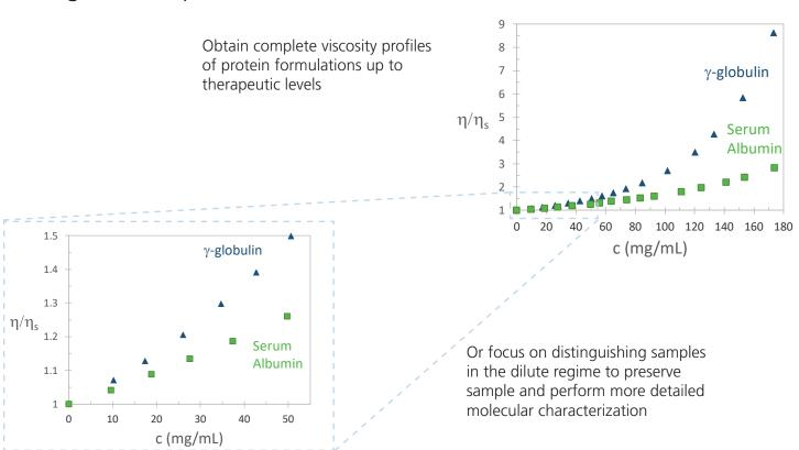
Intrinsic Viscosity Measurement - Detailed Molecular Analysis with
